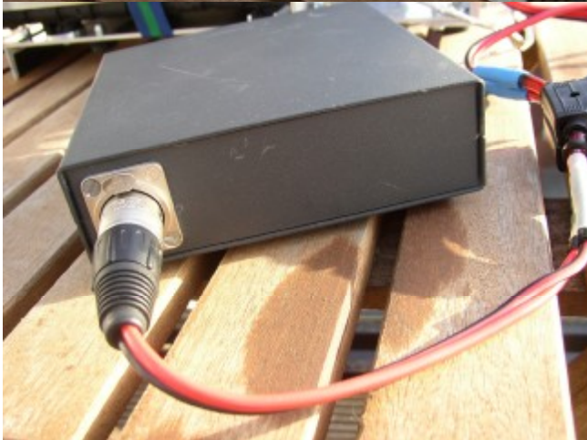
Some power ideas: Double NiMH pack. The second power outlet is situated on the back side.
